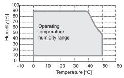
**\*3.** Store the Programmable Terminal within the following temperature and humidity ranges.
